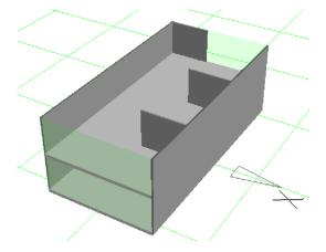
Figure 2. A two-story house with confined masonry walls and concrete roof slab (not shown). Two long boundary walls resist shaking in the direction of the building length. Three shorter walls resist sideways shaking (X-direction). Columns and partition walls are not shown.
