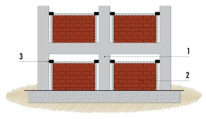
Figure 5. A reinforced concrete frame with potential short columns (1) and masonry infill walls (2) confined by tie columns and tie beams. The infills are separated from the frame by vertical separation gaps but restrained at their top corners by steel brackets bolted to the columns (3). The brackets allow movement between columns and walls parallel to the walls, but prevent the walls from falling from the building during an earthquake.
